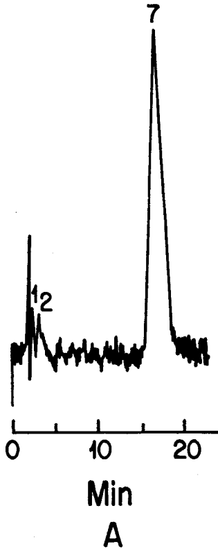
Figure 7. Chromatogram of erythrocyte porphyrins. See Figure 6 for labels. ( Adapted from ref.9 with permission ).
